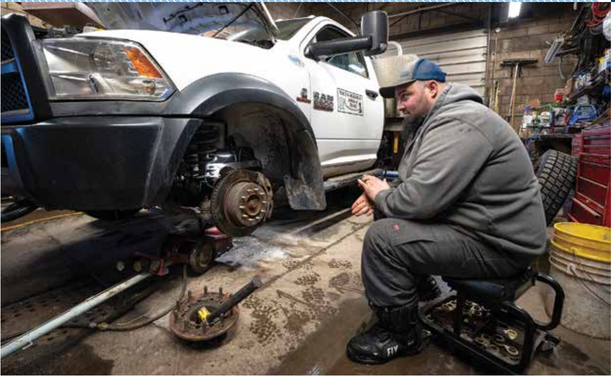
▲ Mechanic Tyler Griffin works to fix the wheel bearing on a service truck. Caring for your fleet of vehicles is an ongoing commitment that requires attention to detail, regular maintenance, and proactive management.
